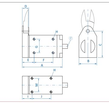
$\bigcirc$  = Compressed air connection 4 mm x 2.5 mm
